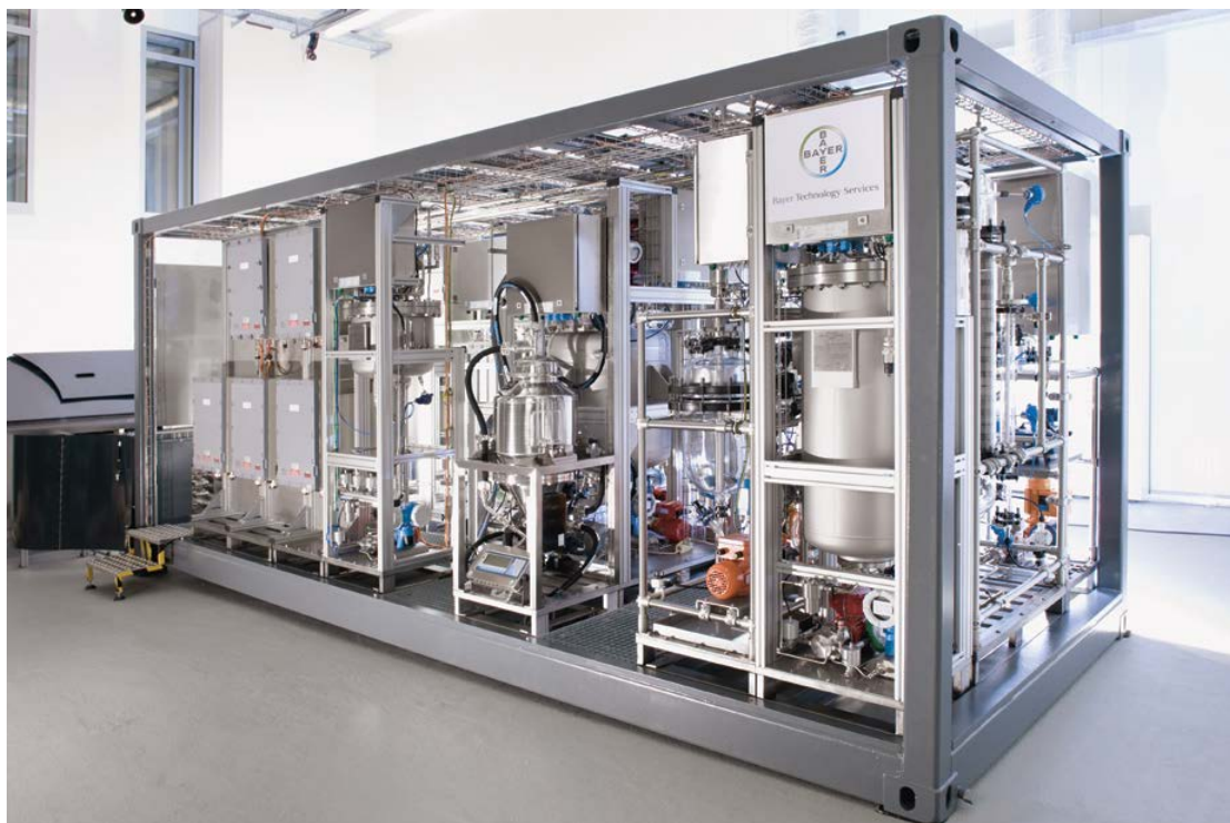
A standardised mini-factory fitted to a transport container. This is the vision of the European research project 'F3 Factory'.
