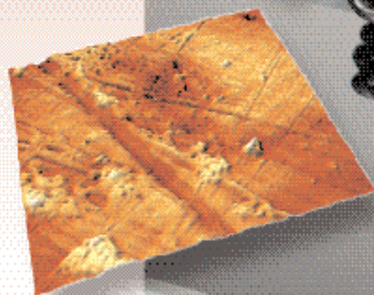
Polish tracks in metal scan size 12 \mu\text{m} z-range 300 nm
